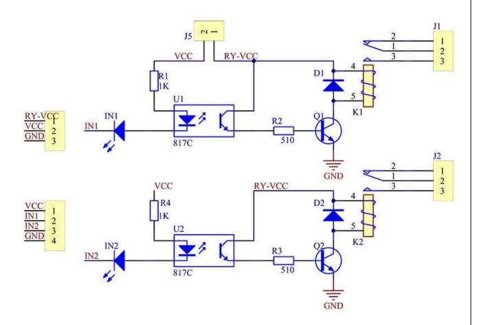
It is sometimes possible to use this relay boards with 3.3V signals, if the JD-VCC (Relay Power) is provided from a +5V supply and the VCC to JD-VCC jumper is removed. That 5V relay supply could be totally isolated from the 3.3V device, or have a common ground if opto-isolation is not needed. If used with isolated 3.3V signals, VCC (To the input of the opto-isolator, next to the IN pins) should be connected to the 3.3V device's +3.3V supply.
